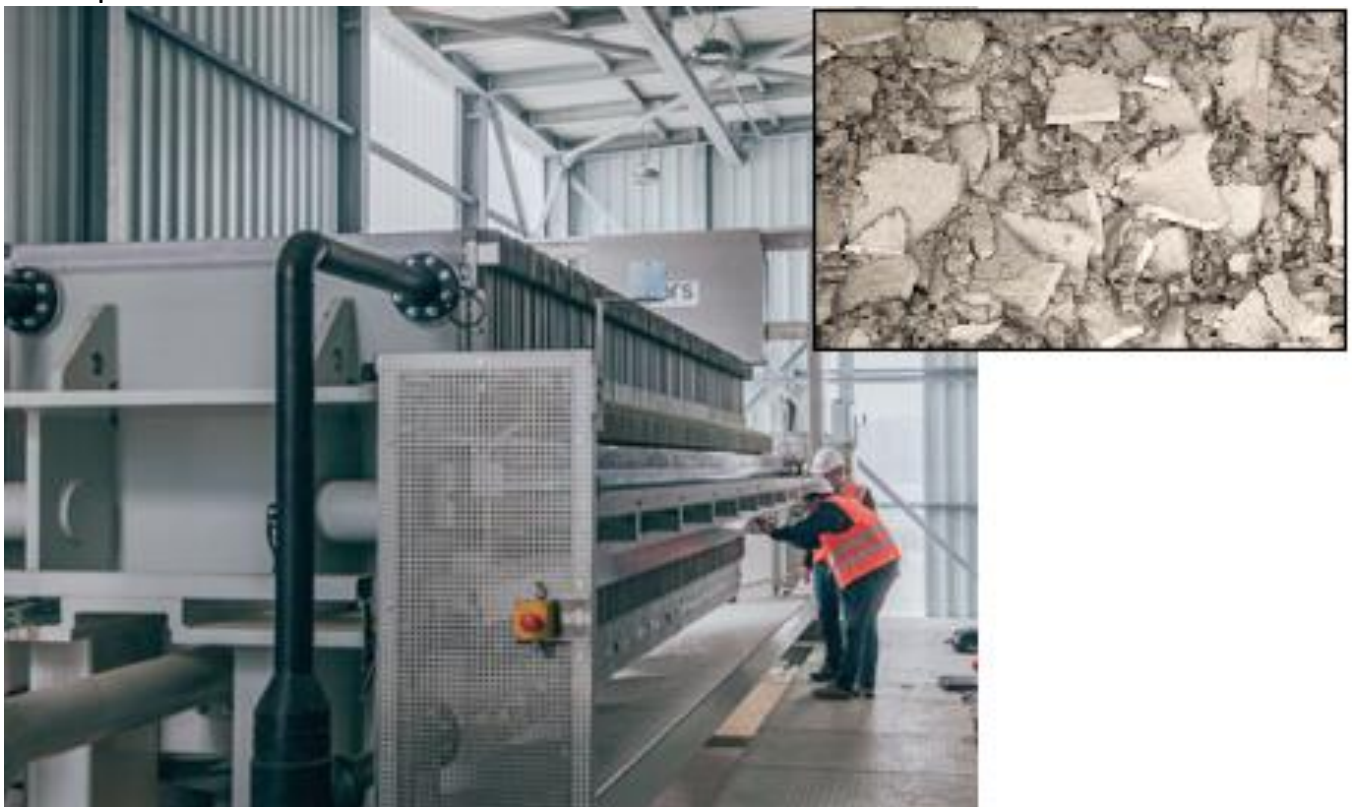
Figure 5: Chamber press, the small picture shows the filter cake, Copyright: ARGE AUDI IN-Campus GbR.
