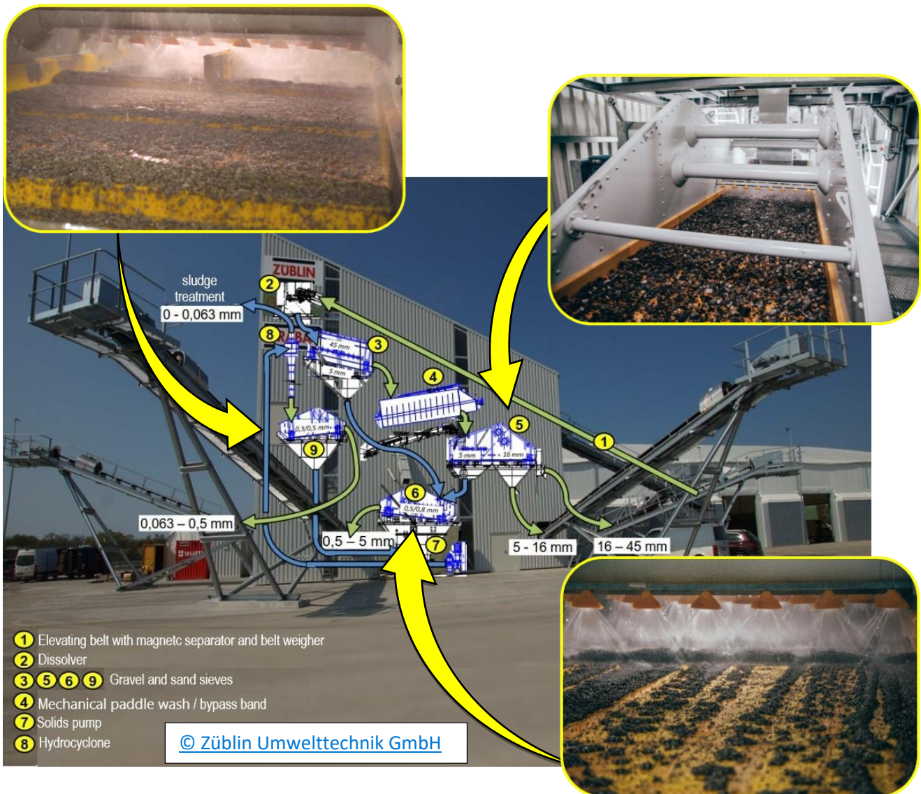
Figure 3: Treatment steps of the soil washing plant.
