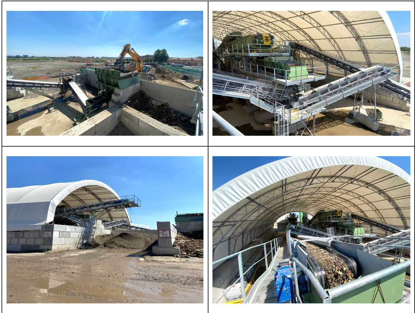
Figure 2.2- Soil washing process (photos by Massimiliano Confalonieri)
