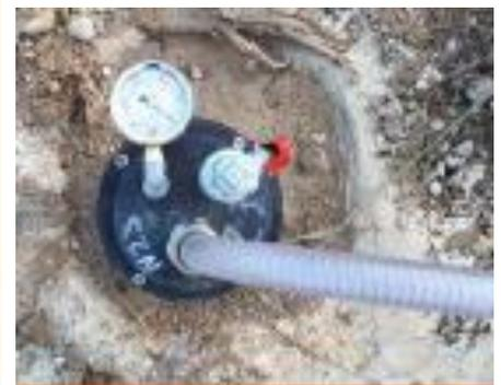
All the well heads, positioned above ground in order to facilitate connections and controls, are equipped with a vacuum gauge to control the depressions induced inside the well and a point of taking samples/measurement with portable instrumentation.
