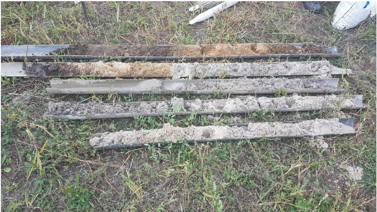
Drill core borehole (sonic drill)
