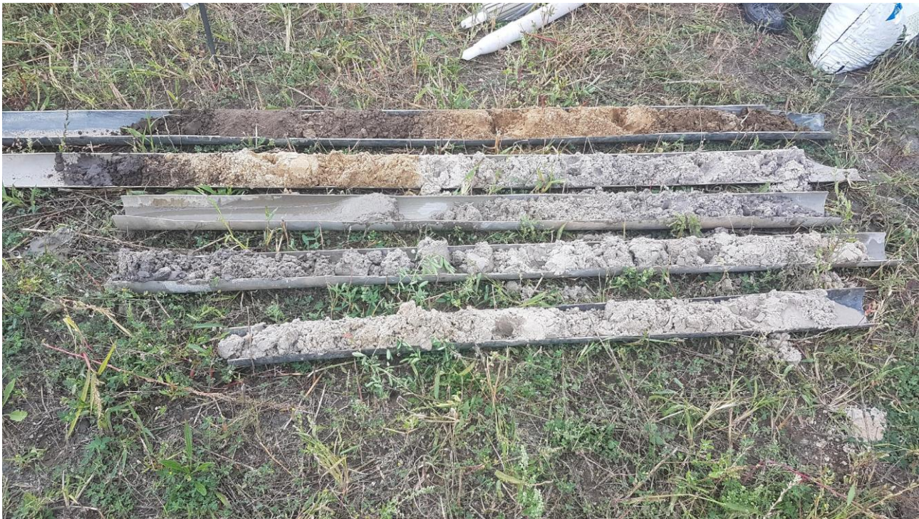
Drill core borehole (sonic drill)
