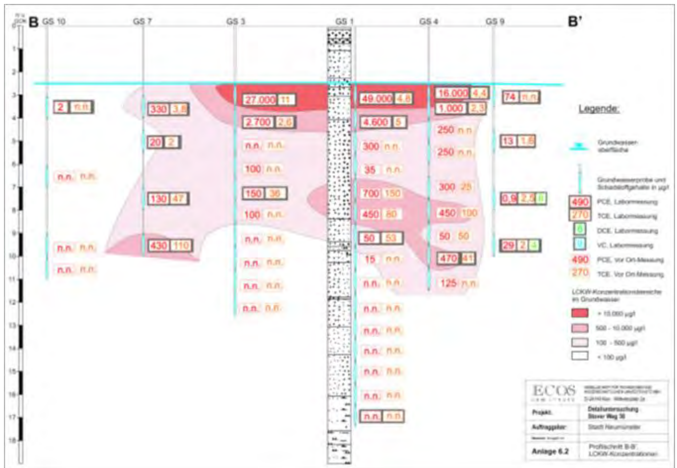
Figure 2: Vertical distribution of pollutants in the contamination centre, source: ECOS Umwelt Nord GmbH
