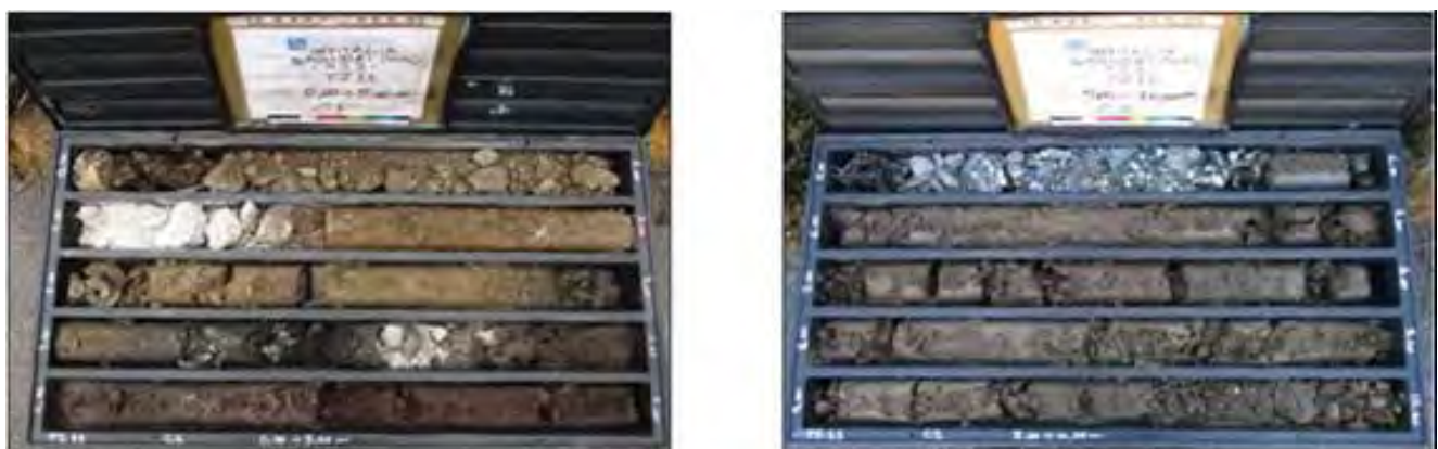
Figure 3 - Typical stratigraphy of the industrial site: fills on volcanic ash
