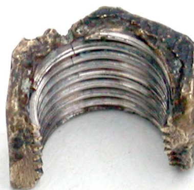
Fig. 8. Piece of the defective nut
