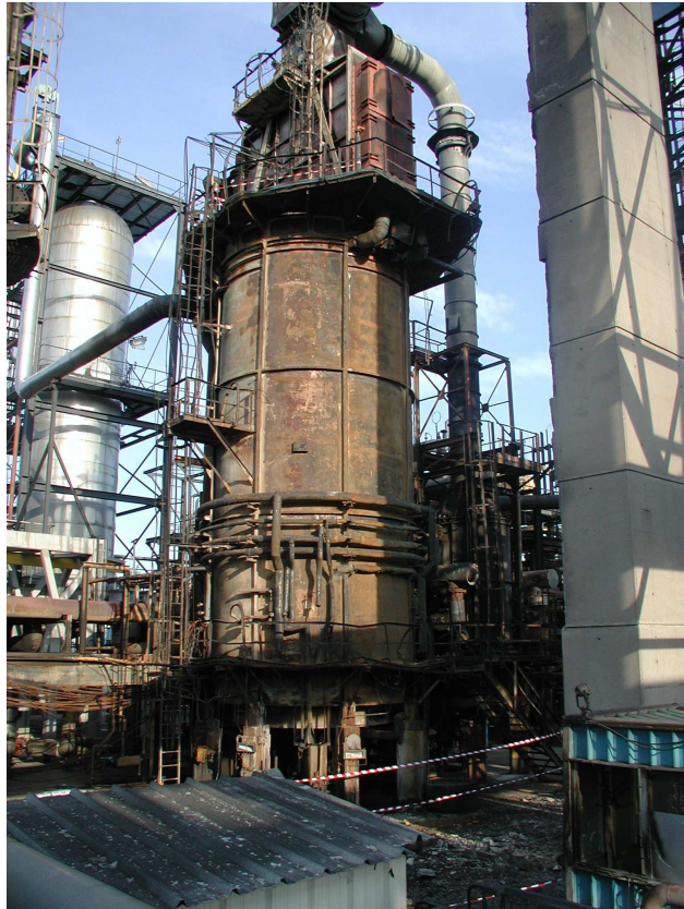
View of furnace 42F201 (after the fire)
