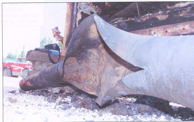
Views of the ruptured tube
