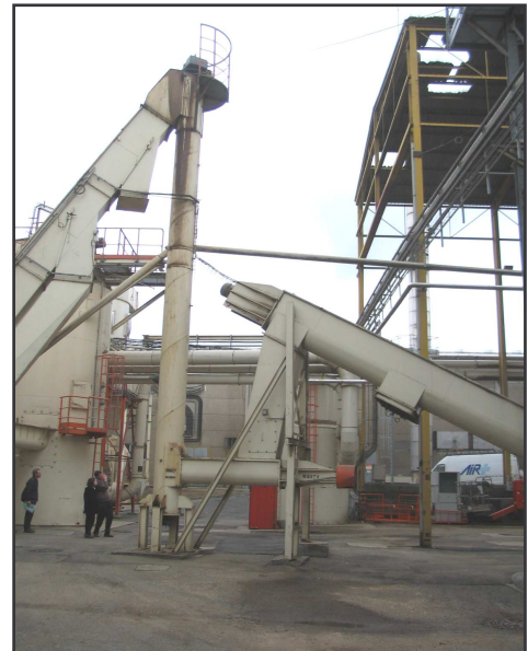
Mechanical transport with decoupling by screw
