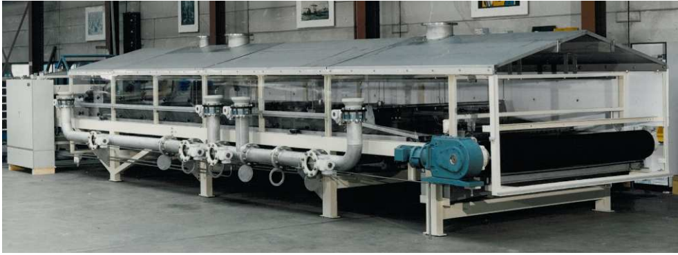
Generic illustration of a RT vacuum belt filter (Picture Larox Pannevis R.R.)
