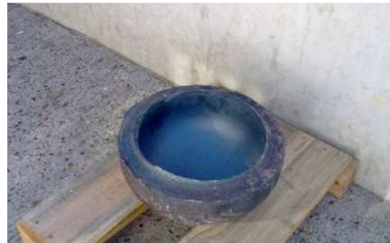
Figure 4 : Photograph of the dished bottom projected on the day of the accident (source: GPN)
