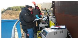
**Figure 4.3** Continuous Emission Monitoring System (Credits: Sardinian Environmental Protection Agency)
