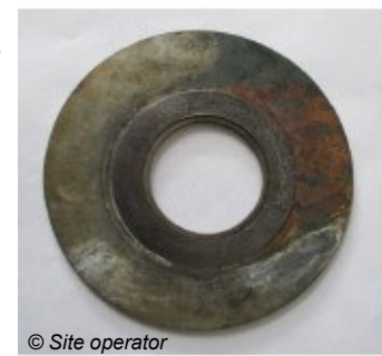
© Site operator Flange's seal upline of the flow meter
