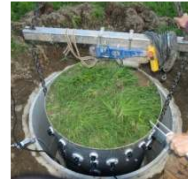
weighable monolith lysimeter
