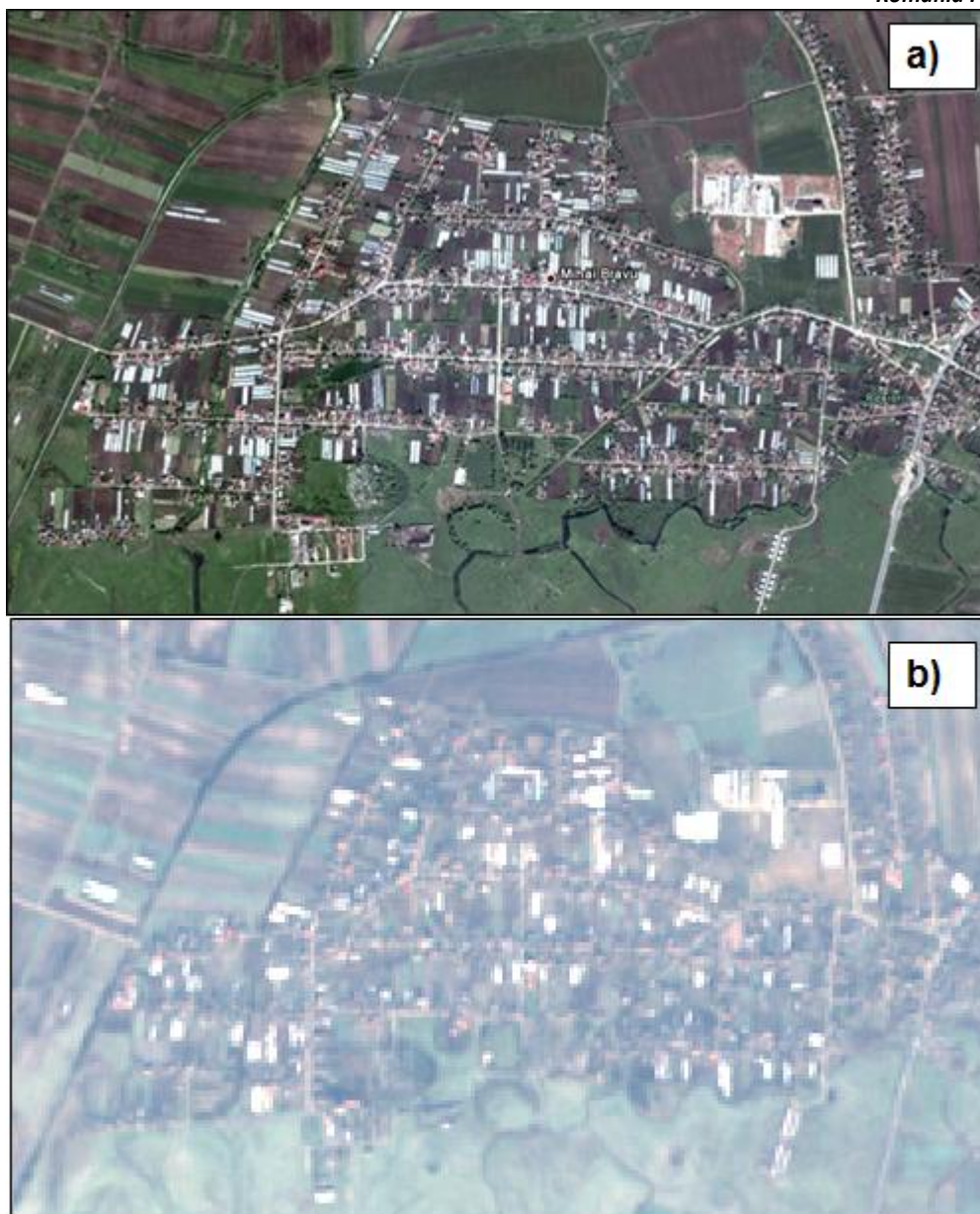
Figure 15: Mihau Bravu area, Bihor County. Comparison between high resolution satellite image available in GoogleEarth (a) and a very recent Sentinel2 image (1 January 2016) at 10 meters resolution (b).
