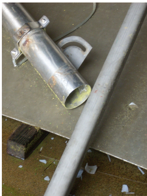
Metal debris, from the pipe blasted by the explosion, found on the floor. The picture on the left shows residue from pyrotechnic dust (yellowish) covering the inner pipe wall.
