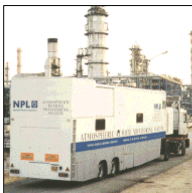
Figure 2.6 - Example of a mobile DIAL measuring vehicle [NPL].
