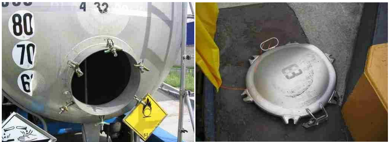
Burst manhole cover (Photos courtesy of the site operator)
