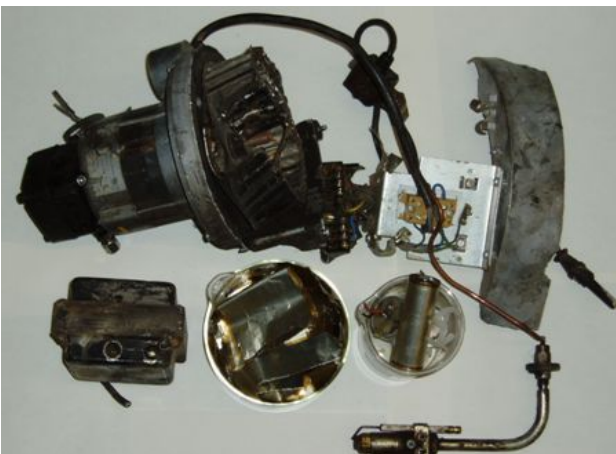
Electric motors with hazardous substances
