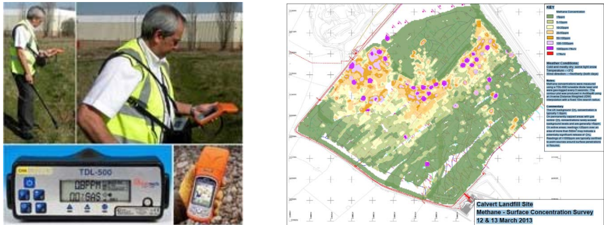
Figure 22: Methane walk-over surveys
